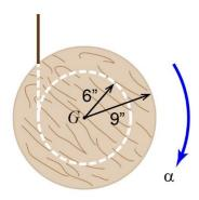
Calculate the spool's mass moment of inertia.
